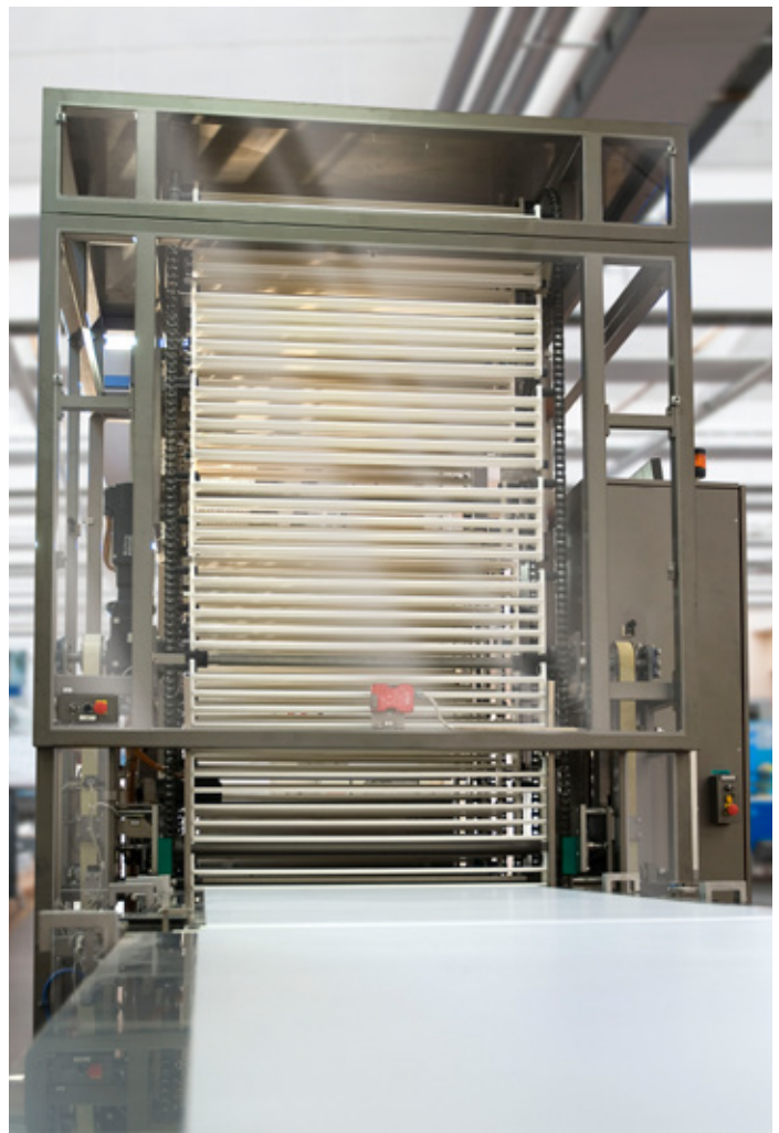
Vertical buffers can optimize feeding and mitigate time lost to microstops.
